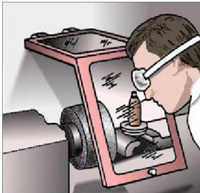
LATHE. Worker protected by guard and personal protective equipment.
