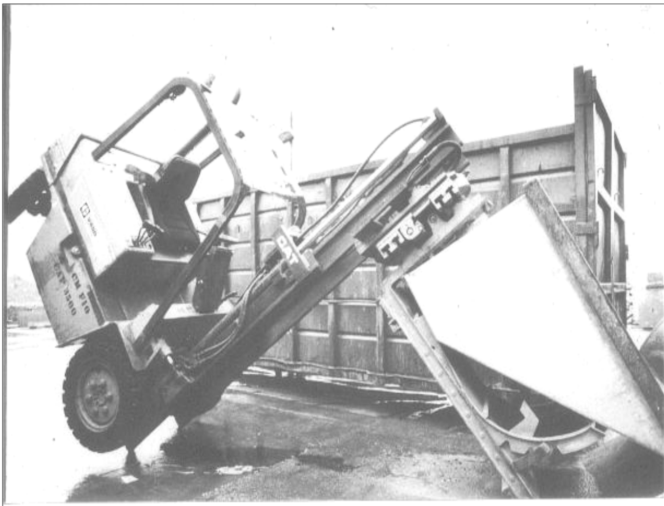
This forklift tipped over because the Center of Gravity moved outside the Stability Triangle
