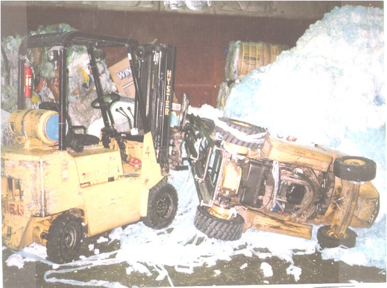
This forklift tipped over because the Center of Gravity moved outside the Stability Triangle
