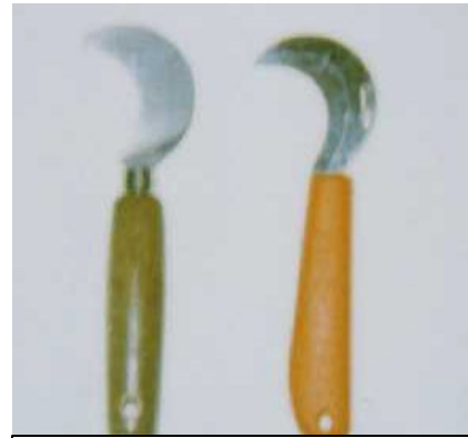
Figure 7: Existing wooden handle (left) and plastic handle (right).
