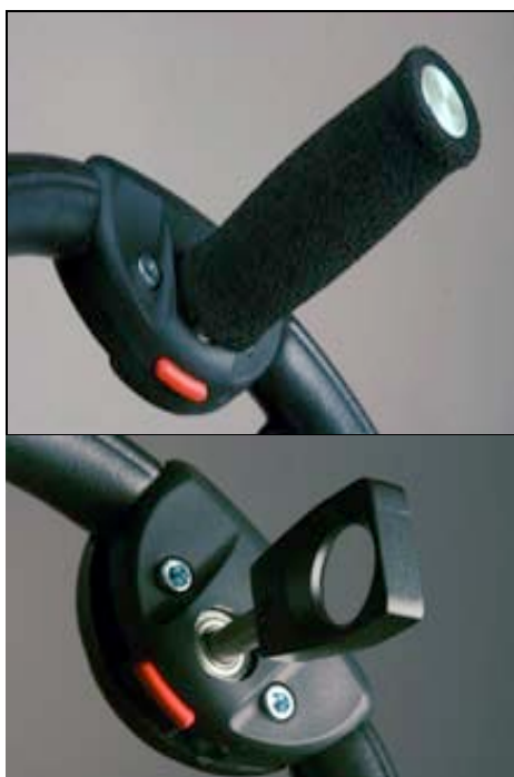
Figures 3 & 4: Grip Knob and Thumb Grip may work well for some farmers ( www.mobilityworks.com )
