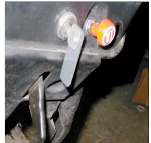
Figure 1: PVC Key Extender (AgrAbility Project Adaptive Controls for Tractors and Machinery, T. Prather, UCCE, U. of Tennessee, 2003)
