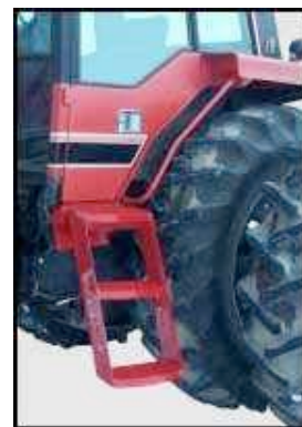
Figure 5: Add-on tractor steps can make mounting large machinery less painful and dangerous ( www.fyi.uwex.edu )
