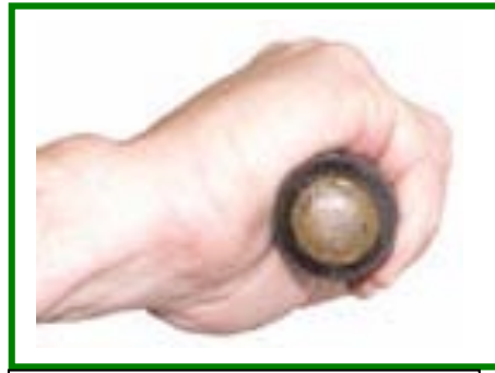
Figure 4: Best handle diameter for power tasks is 1-1/4 in. to 2 in. (Images: NIOSH Pub. No. 2004-164)
