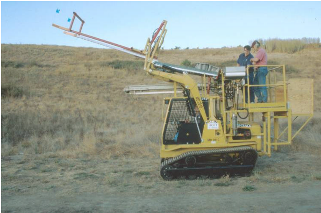
Figure 8. Forks in elevated and tilted position for turning clearance and container transfer.
