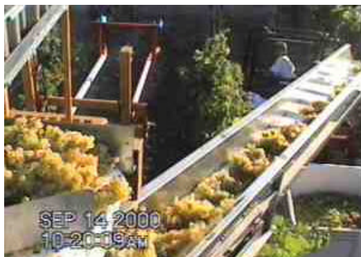
Figure 13. Transfer to discharge conveyor.
