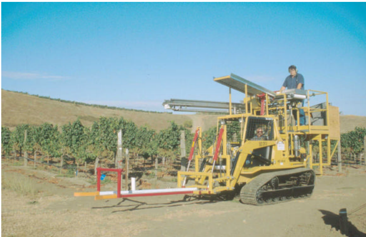
Figure 7. Machine for handling picking containers, with only tractor driver and dump attendant pictured. Third person, designated for sorting would be standing to the right of the dump attendant pictured.
