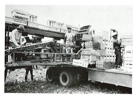
Outdoor automation produces boxes on the spot where the lettuce is grown.
