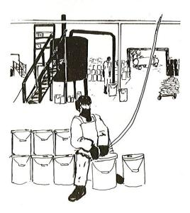
Following manufacture, the active ingredient usually goes to a formulating plant, where it is mixed with other chemicals and a carrier for effective delivery. These are the inert ingredients. They may include such materials as talcs, oils, kerosene, and binding agents (to increase adherence).
